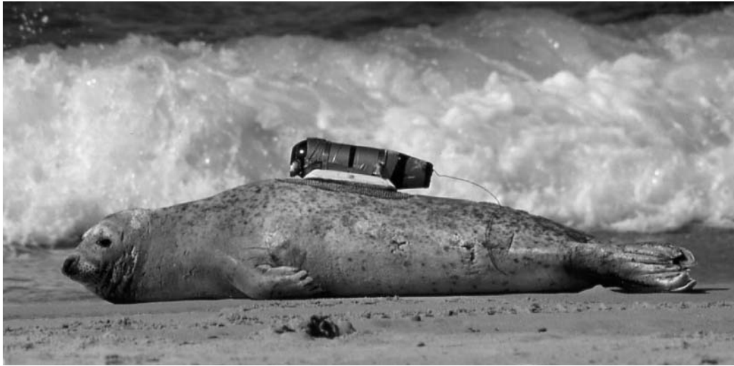
Fig. 1. Phoca vitulina . Crittercam video system used to record foraging behaviour of 39 adult male harbour seals. The tapered cylinder at the rear of the camera is for flotation
